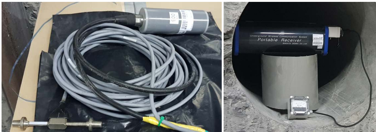
Figure 7-1: Miniaturized transmitter and vibrating wire extensometer (on the left) – Portable Receiver connected to the needle indicator (on the right)
