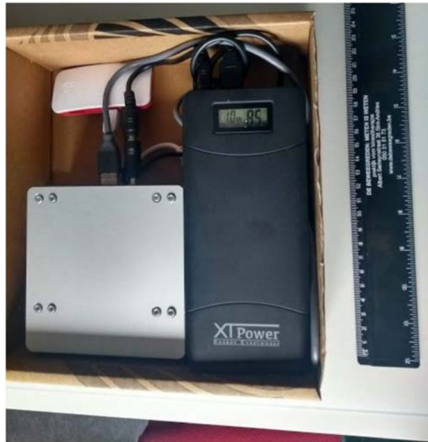
Figure 7-9: Preliminary assembly fits in a box 23 x 21 x 7 cm 3
