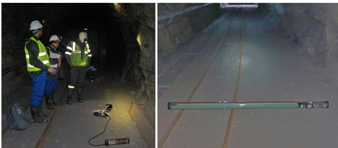
Figure 5-16: Receiver (left) and transmitter (right) used at FSB
