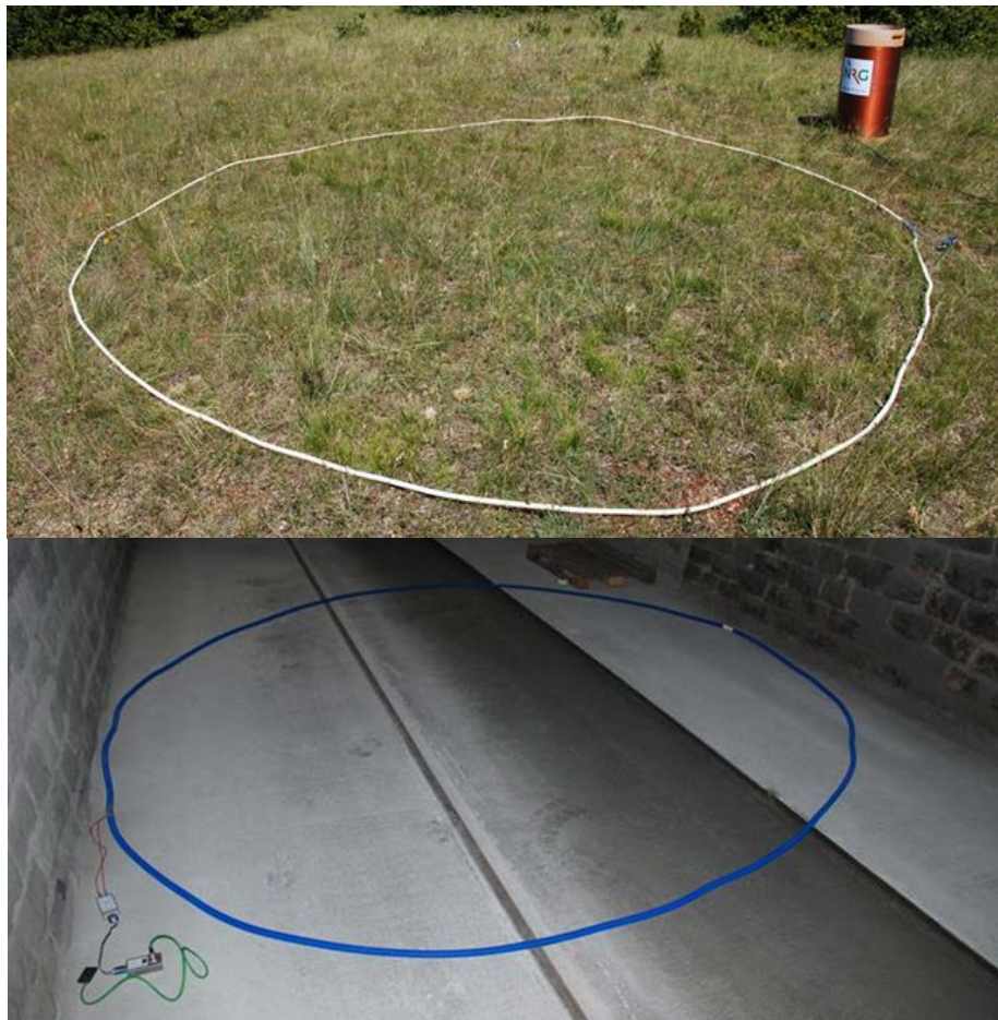
Figure 7-17: Antennas used in Tournemire: Receiver antennas NRG-5 (top left) and NRG-4 (top right), transmitter antenna NRG-6 (bottom)
