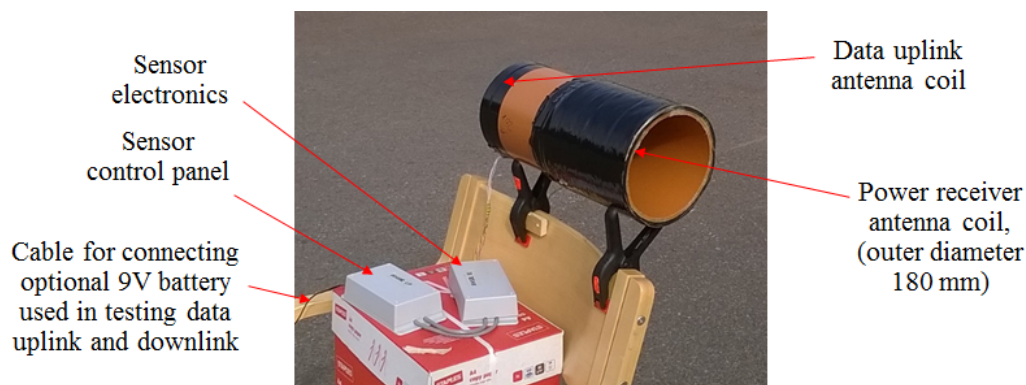
Figure 6-6. The sensor part of the pilot system.
