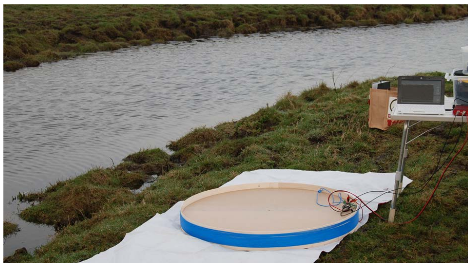
Figure 6-20. Field measurement of antenna impedance in a wet grassland in Ursem, NL.
