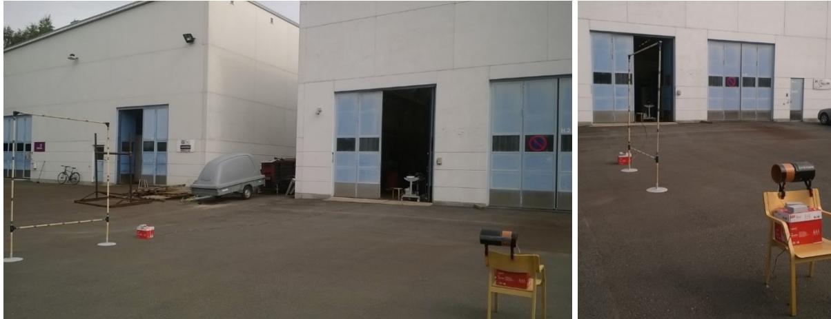
Figure 6-7. The pilot system in co-axial antenna configuration (left) and co-planar antenna configuration (right) through the air at VTT premises in Oulu, Finland.
