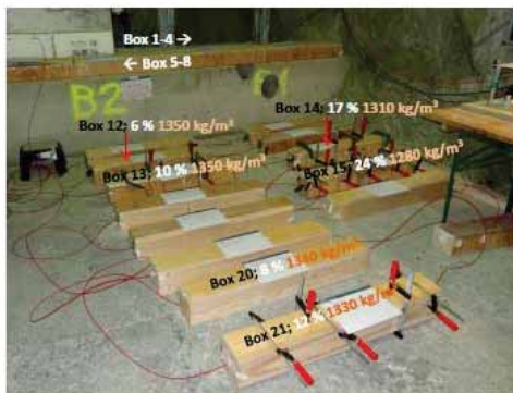
Fig. 5-2: Photograph of the test setup Note: For the higher water content boxes, metal clamps were used to constrain the volume.
