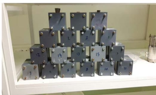
Figure 84. Diffusion cells for wetting compacted bentonite samples. On the right diffusion cell where external water sources are below and above of stainless steel sample holder. Liquid is separated from bentonite sample by sinters.
