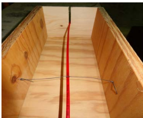
Figure 60: The FO cable fixed along the centerline of the test box
