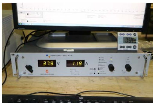
Figure 57: Electrical current generator
