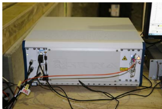
Figure 55 : The main DTS unit. Silixa Ultima-S (Silixa Ltd. 2015[103])
