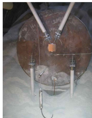
Figure 71: Extensometers (white pipes) installed in FE experiment
