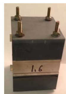
Figure 84. Diffusion cells for wetting compacted bentonite samples. On the right diffusion cell where external water sources are below and above of stainless steel sample holder. Liquid is separated from bentonite sample by sinters.
