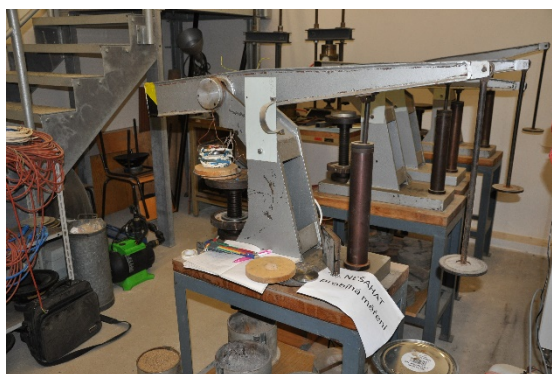
Figure 102: First prototype test in press (heat toleration test in progress
