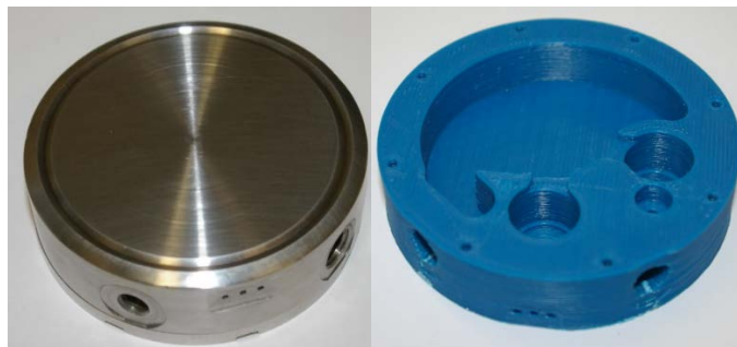
Figure 101: (On the left) First body version of smart cell (stainless steel body; (on the right) 3D printed prototype
