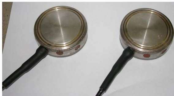
Figure 105: 2nd revision smart cells (cell on the left designed for LTRBM)
