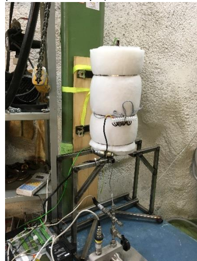
Pressure test system with heating(Max pressure 20Mpa)
