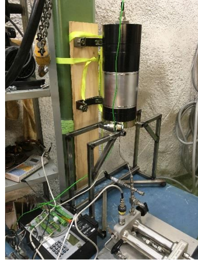
Pressure test system with heating(Max pressure 20Mpa)
