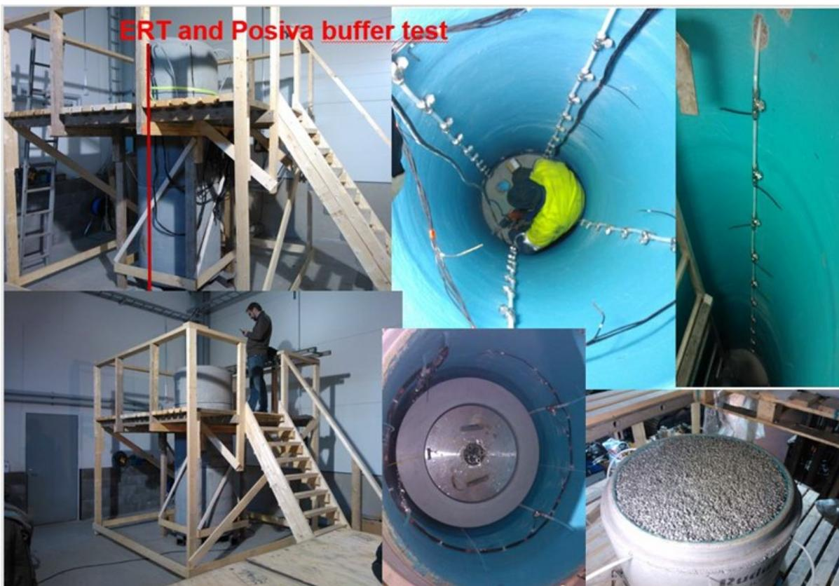
Figure 8.1. The ERT mock up test set up for the experimental 40%-scale bentonite buffer - canister structure
