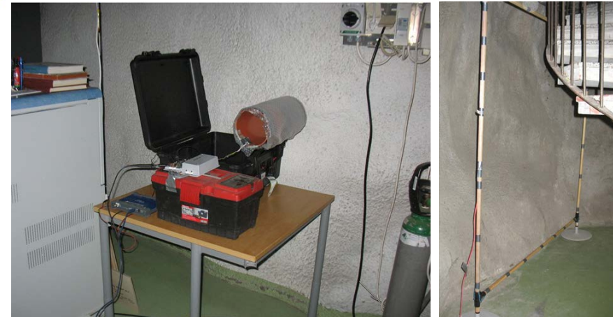
Wireless energy transfer pilot system with integrated communication add-on through crystalline host rock in Finland by VTT
