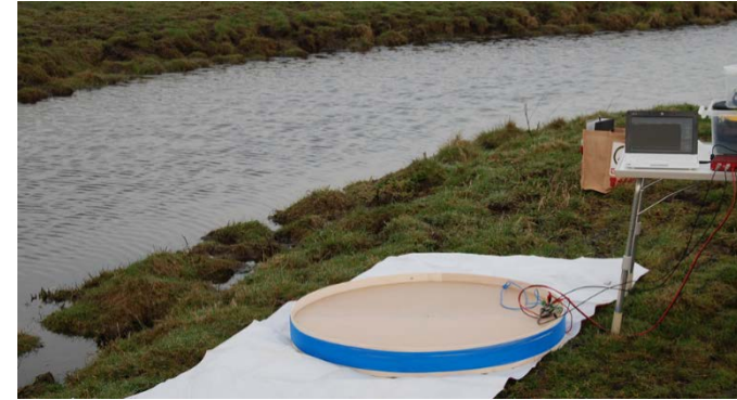
Wireless energy transfer pilot system in wet grassland in the Netherlands by NRG
