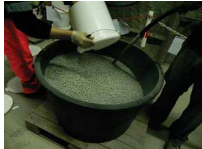
Charging of the screw conveyor tank with GBM
