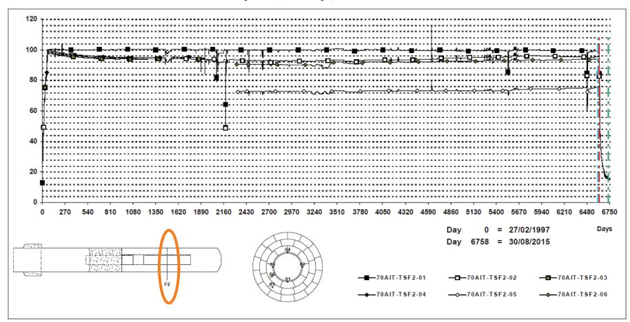
Blue: the start-up of the plug dismantling (day 6614) dashed vertical lines: Red: the heater switch off (day 6630) Green: the end of the dismantling operation (day 6758)
