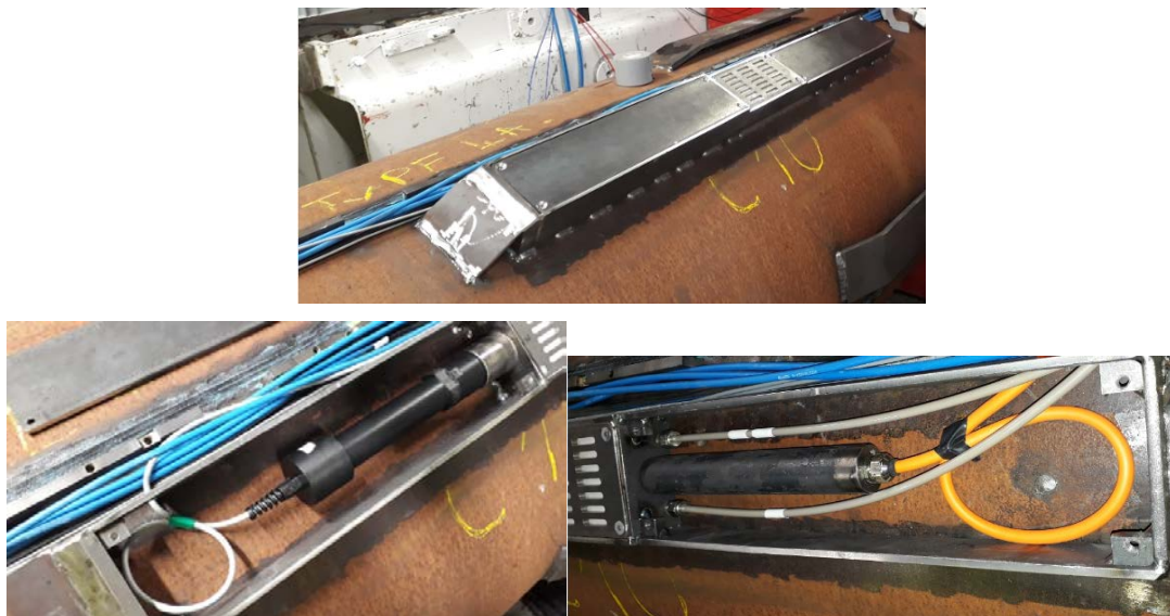
Figure 55: Some picture of the instalaltion of the H2 et O2 sensors on the sleeves n°10 with Peek lines for future comparative measurement
