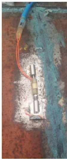
Figure 53 : Picture of the Geokong vibrating wire sensor 4150 on the sleeve before the installation of the protection system
