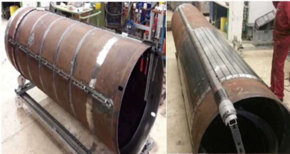
Figure 30: picture of the sleeve n°52 without (left) and with metal protection plate .
